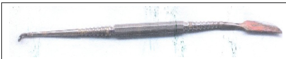
Lecron. Note blade at one end and rounded termination at other.
